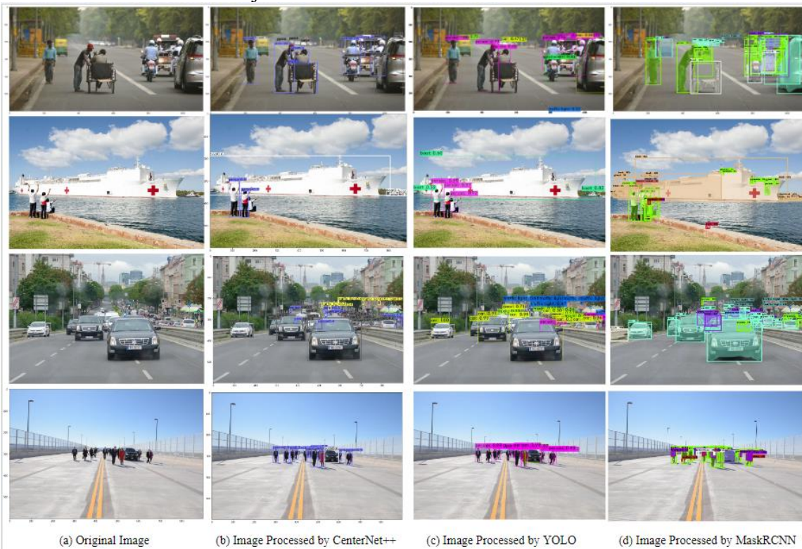
Figure 2. A comparison of the sample image and the processed image by CenterNet++, YOLO, and MaskRCNN.
